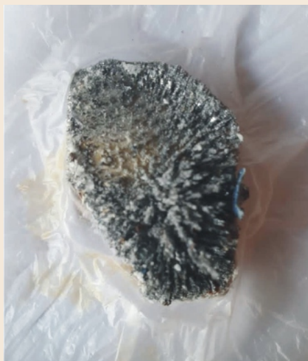
Metallic contaminants extracted from (a) wet maize, and (b) dry maize, using regular milling machine
