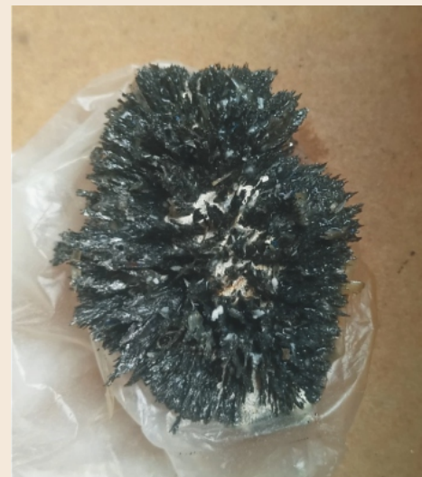
Metallic contaminants extracted from (a) wet maize, and (b) dry maize, using regular milling machine
