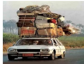
Figure 6: Unsafe loading ignorance
