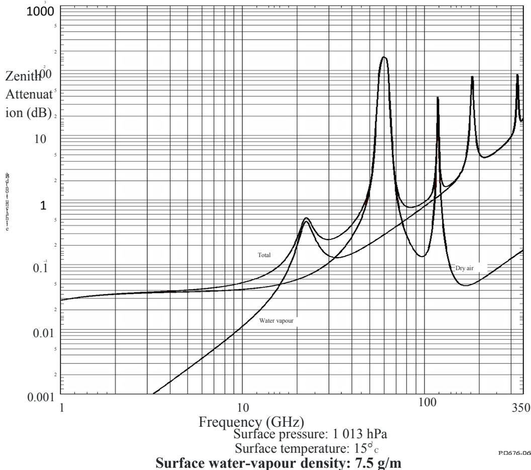
**Fig. 5: Atmospheric gases contribution to zenith attenuation**
