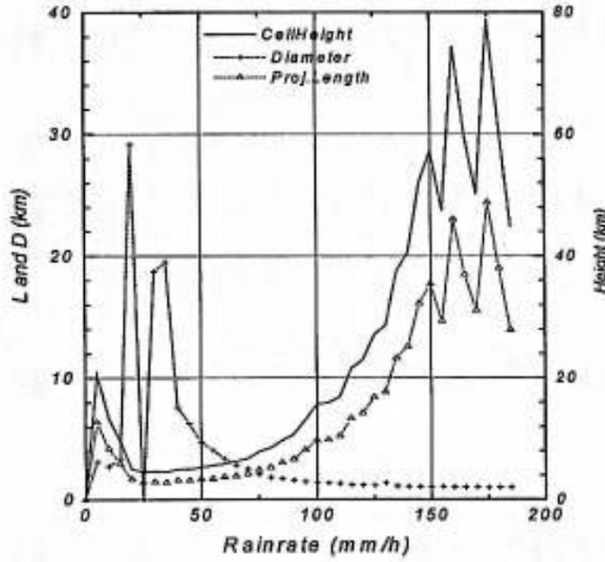
**Fig.15: projected path length, cell diameter and attenuation exceedances**
