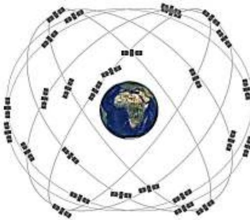
**Fig. 3: GPS satellite constellation flying in the Medium Earth Orbit (MEO)**
