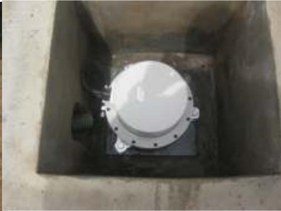
The magnetometer sensor
