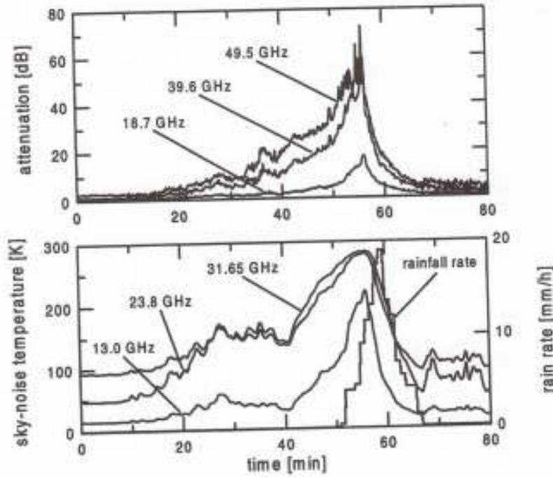
**Fig. 18: ITALSAT Sample attenuation, radiometric and rainfall rate data**
