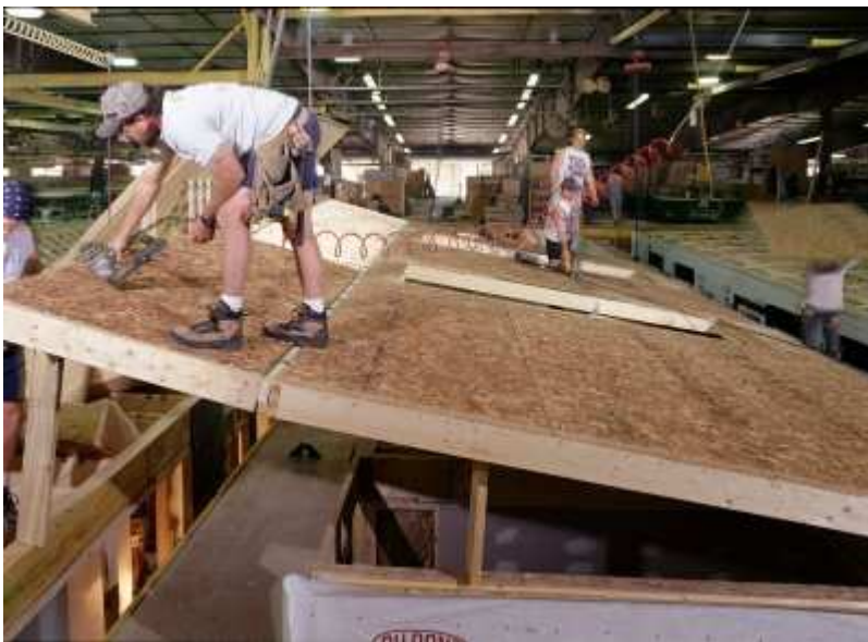
Figure 16. Home Factory Picture showing workers performing work on the ceiling and on a hinged roof of a module
