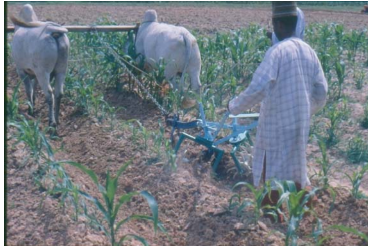
Figure 37. Inter-row rotary weeder showing proper alignment with the side slopes of adjacent ridges.
