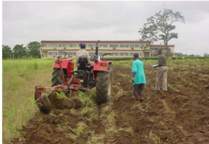
Figure 12. Measurement of implement depth-of-cut during field evaluation of a tractor.
