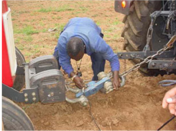
Figure 14. Coupling of the dynamometer for draught force determination.
