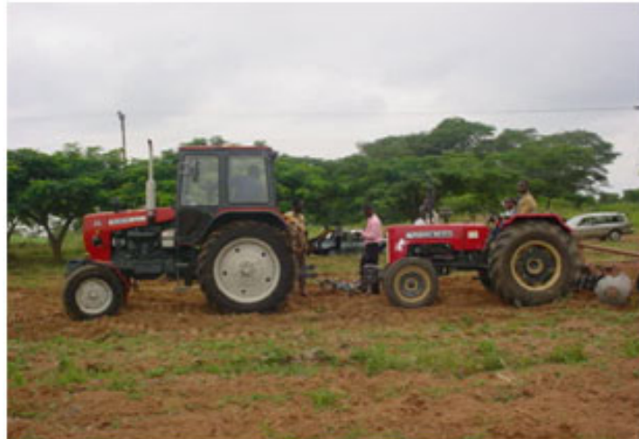
Figure 13. Measurement of tractor draught using a 20 kN Strain gauged dynamometer.
