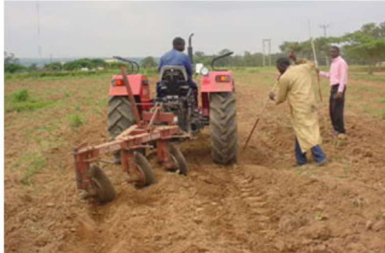
Figure 10. Slippage determination during field evaluation of a tractor.
